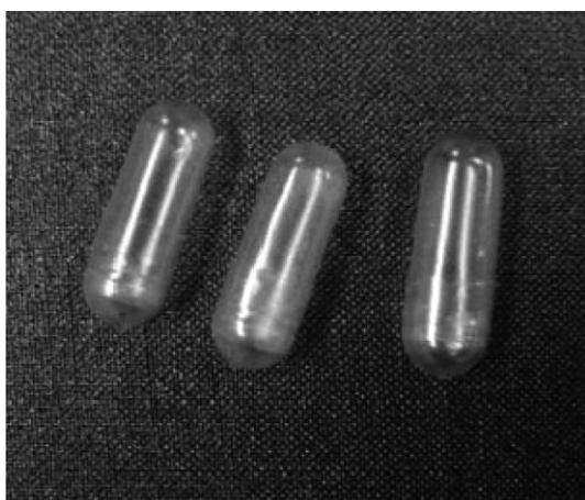
Fig. 7. Waterchestnut starch hard capsule without gelling agent.
