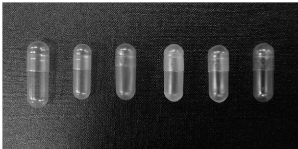
Fig. 5. Developed starch capsules: (a) HPMC capsule, Suheung capsule, Korea; (b) HPMC capsule, Capsugel, France; (c) sweet potato starch capsule; (d) potato starch capsule; (e) mungbean starch capsule; and (f) waterchestnut starch capsule.
