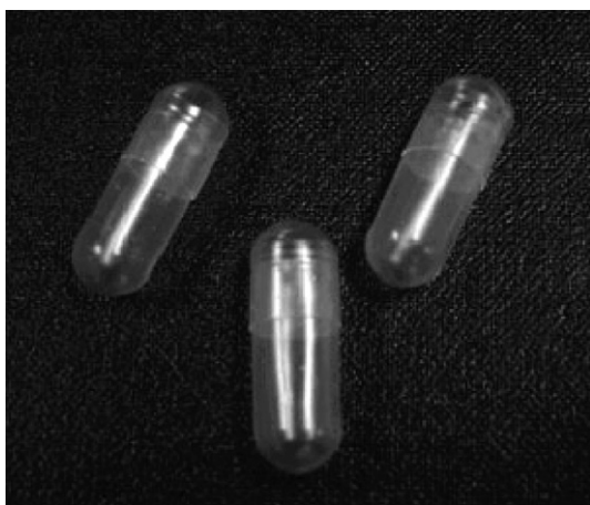
Fig. 6. Mungbean starch hard capsule without gelling agent.
